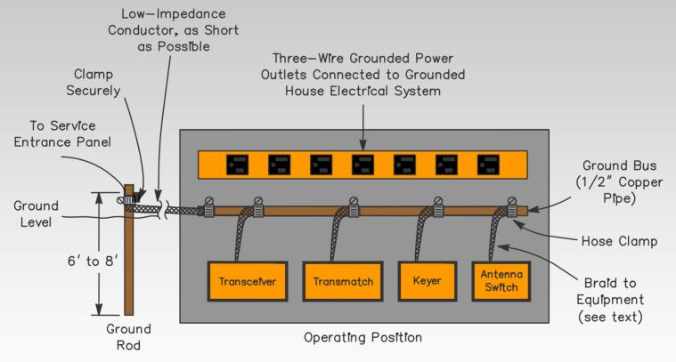
For best protection from electrical shock all equipment should be connected to a common ground.
